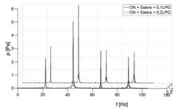
Fig. 10. Amplitudinous spectrum of acoustic pressure measured in proximity of cylinder head with addition of LPG to mixture of diesel oil and ester oil with LPG
