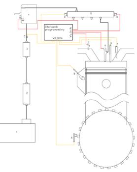
Fig. 2. Workbench diagram: 1-container, 2-electric pump, 3-fuel filter, 4-high pressure pump, 5-
